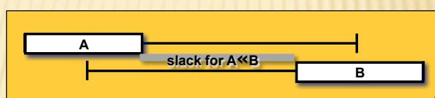
$$\text{slack}(A \ll B) = \max(\text{end}(B)) - \min(\text{start}(A)) - p(\{A, B\})$$
